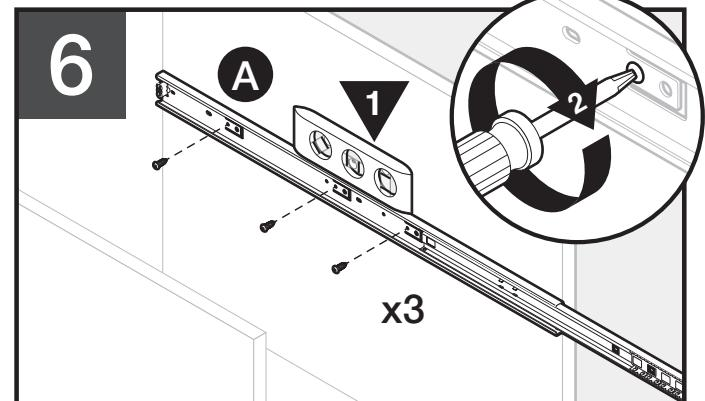
Make sure cabinet member (A) is level; secure with screws (D). Repeat Steps 5-6 for remaining cabinet member (A). Insert drawer into cabinet and close. Release lever (B) will lock.
