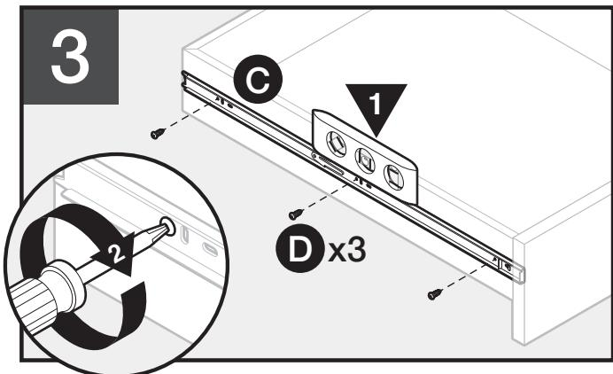
Make sure drawer member (C) is level; secure with screws (D). Repeat Steps 1-4 for remaining drawer member.
