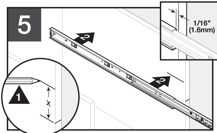
Mark "X" from bottom of mark. Align top of cabinet member (A) with mark, 1/16" from front of cabinet.
