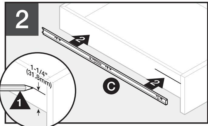
Mark 1-1/4" (32 mm) from bottom of drawer. Align top of drawer member (C) with mark.
