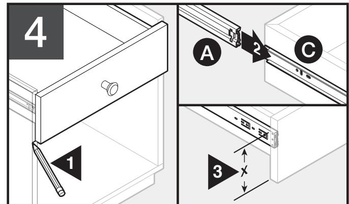
Determine drawer position. Mark bottom of drawer front. Place cabinet member (A) onto drawer member (C). Measure "X".
