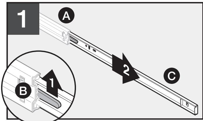
Press release lever (B). Remove drawer member (C) from cabinet member (A).
